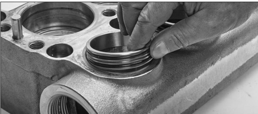
2.30 Install inlet spacer in each seal chamber.
