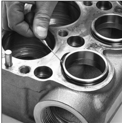
2.6 Use a pick to remove o-ring from top of inlet spacer.
