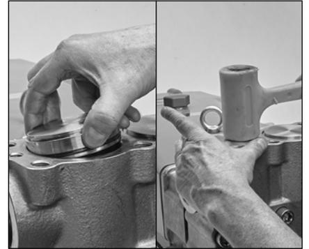
1.12 Install valve plug by hand and then tap with a rubber hammer to seat properly.
