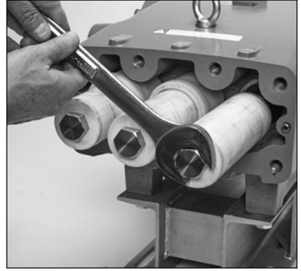
2.33 Use a M30 hex wrench to loosen the plunger retainers.
