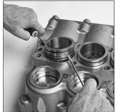
2.4 Insert two (2) flat tip screws into the groove on opposite sides of v-packing spacer and pry upward.
