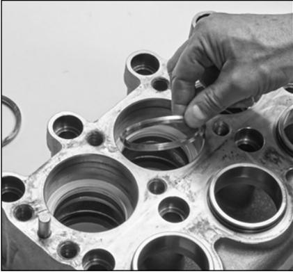
2.16 Remove male adapter from each seal chamber.
