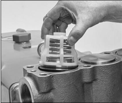
1.9 Place new preassembled valve assembly into each valve chamber.
