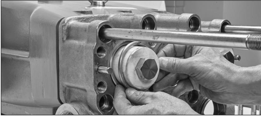
2.51 Install large coil spring over each ceramic plunger and press into place.
