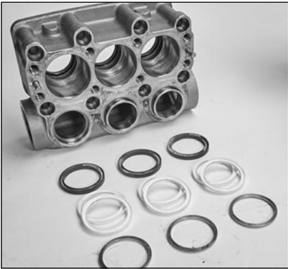
2.19 V-Packing assembly arrangement.
