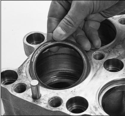
2.24 Install female adapter in each seal chamber with flat surface facing down.
