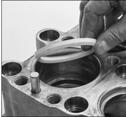
2.25 Install the pair of v-packings in each seal chamber with v-shape facing down.
