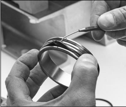
2.8 Use a pick to remove o-ring from the one end of the inlet spacer.
