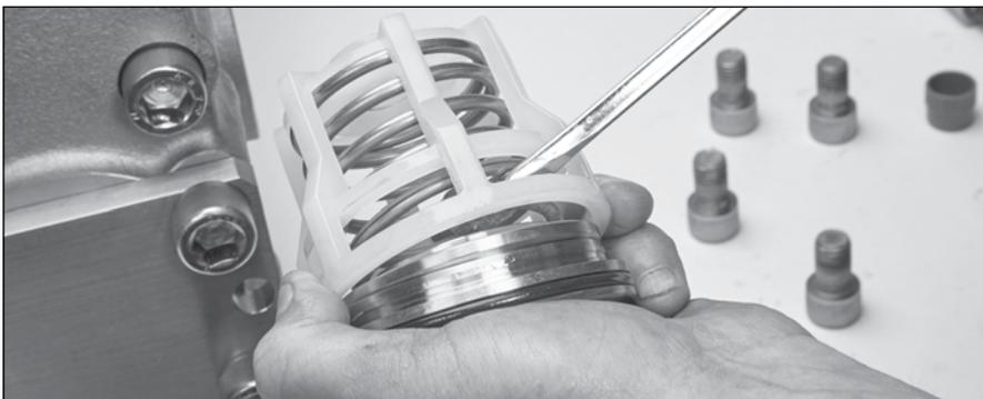
1.6 To separate spring retainer from valve seat, insert a flat tip screw driver between spring retainer and top of valve and pry upward until there is small gap.
