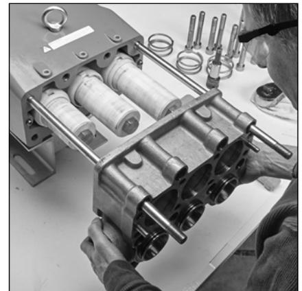
2.15 Remove inlet manifold and place on work surface with crankcase side down.
